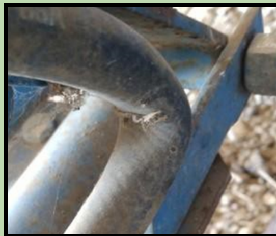
Figure 1. Crimps in hoses may lead to cracking (Photo: Ric Bessin, UK).
